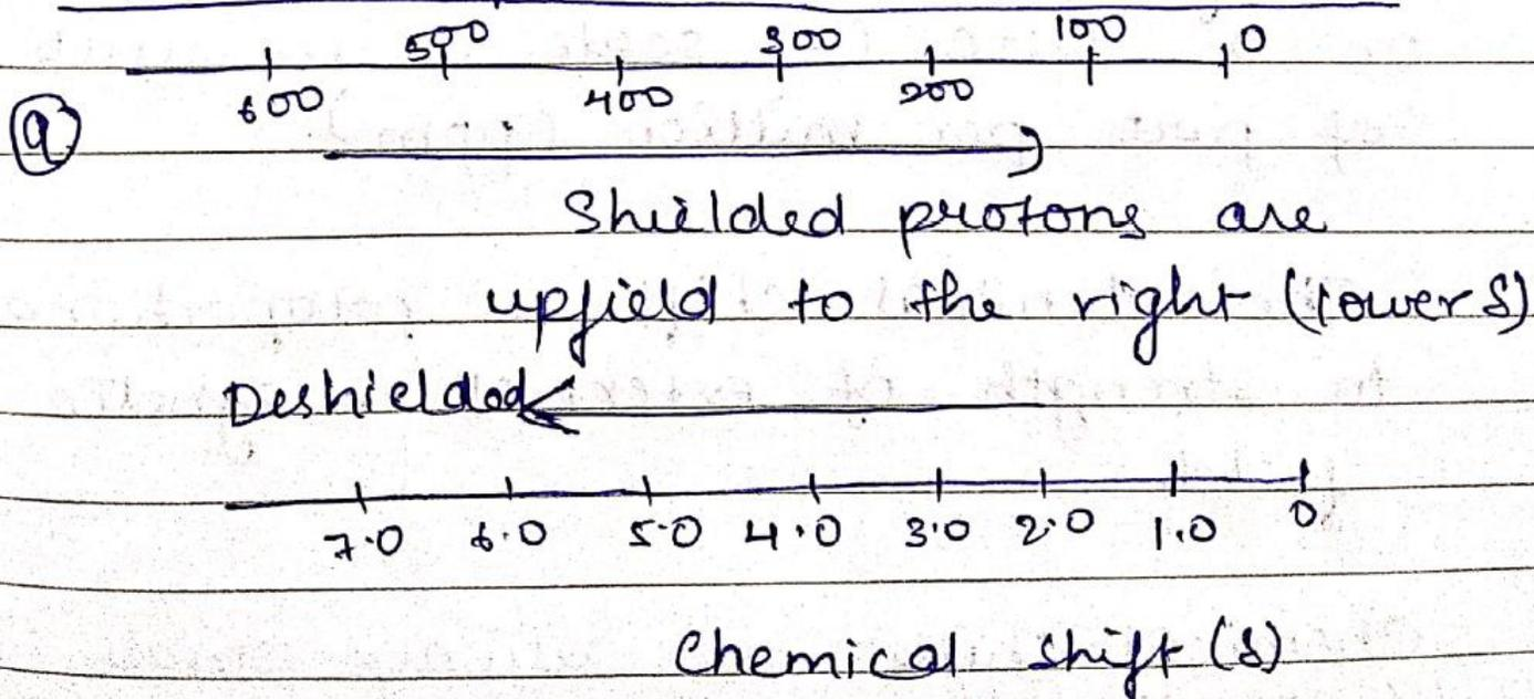
The reference  $\delta = 0$  is for Tetra methyl silane. The TMS is the internal standard for the sample.
