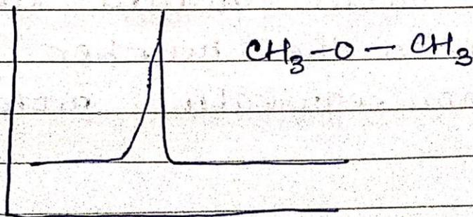
All the six hydrogen atoms are in the same environment and therefore show only one sharp signal.
